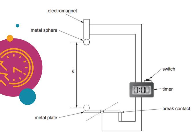
When the switch is pressed, it starts the timer and disconnects the electromagnet, almost instantly releasing the metal sphere. When the sphere hits the metal plate it breaks the circuit, stopping the timer. The time taken for the metal sphere to fall through a range of different heights, h is measured.
