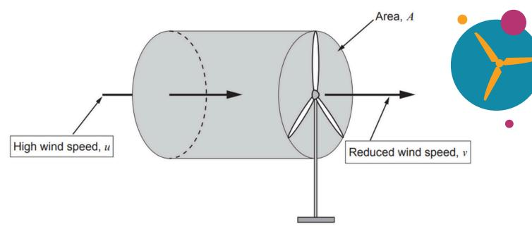
(a) (i) The volume of air arriving on the blades per second is *Au*. Show that the kinetic energy per second (the power, *P*) arriving is given by:
