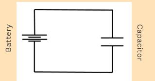
As one plate becomes more **positively** charged, it becomes **harder to remove the negative electrons** from it, just as it becomes harder to **add** them to the negatively charged plate. The **rate of flow of charge (current)** therefore depends on the **charge of the capacitor** - this is an **exponential relationship**:
